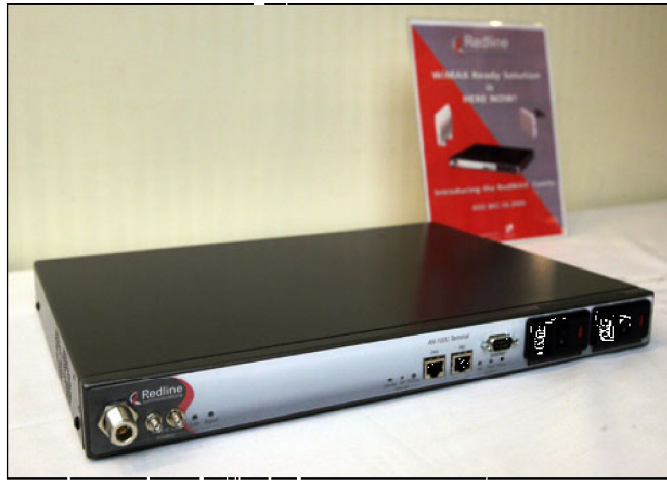
WiMax base station Redline Communication's WiMax access point (Fig a)
